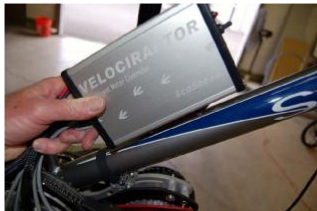
(19) Mounting Controller on Bracket
