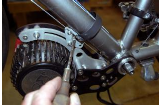
(9) Installing Band Clamp
