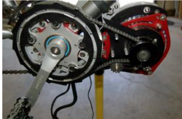
(15B) Motor Chain Installed
