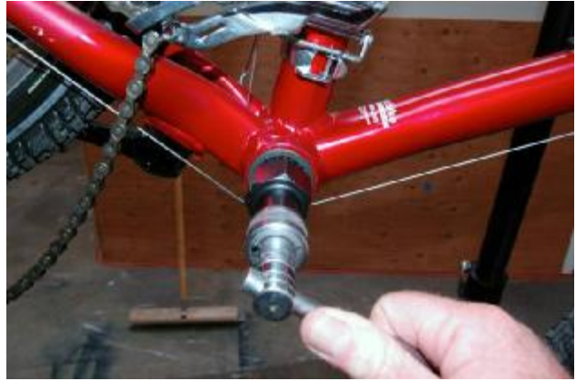
(3) Removing Bottom Bracket
