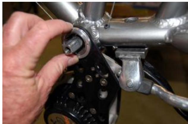
(7) Unit Hanging from Left Ring. Installing Left Lock Nut
