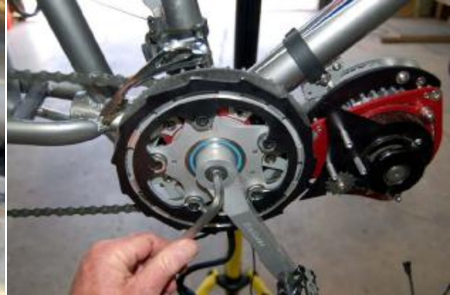
(13) Installing Crank Set
