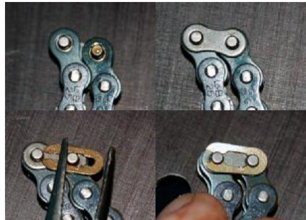
(15A) Installing Master Link (clockwise from top left)
