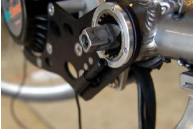
(12) Cadence Sensor Installed
