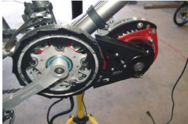
(17) Motor Chain Cover Installed
