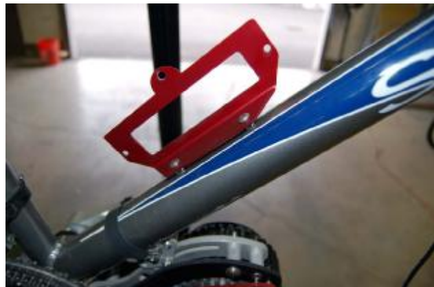
(18) Bracket for Attaching Controller to a Water Bottle Mount
