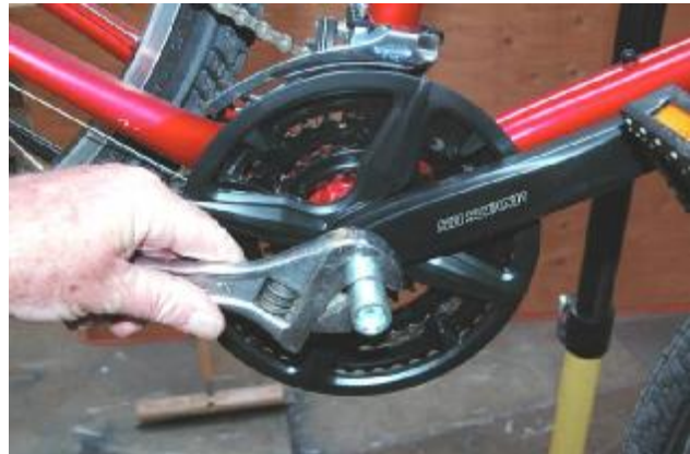
(2) Removing Crank with Crank Puller
