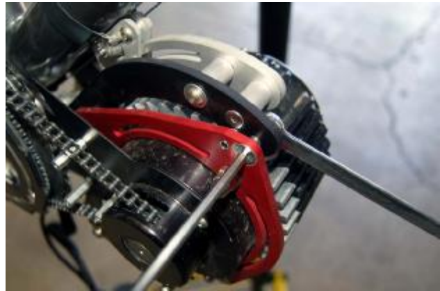
(16) Loosening Adjust Plate Bolts
