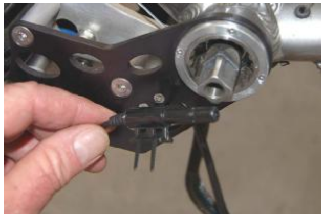
(11) Installing Cadence Sensor
