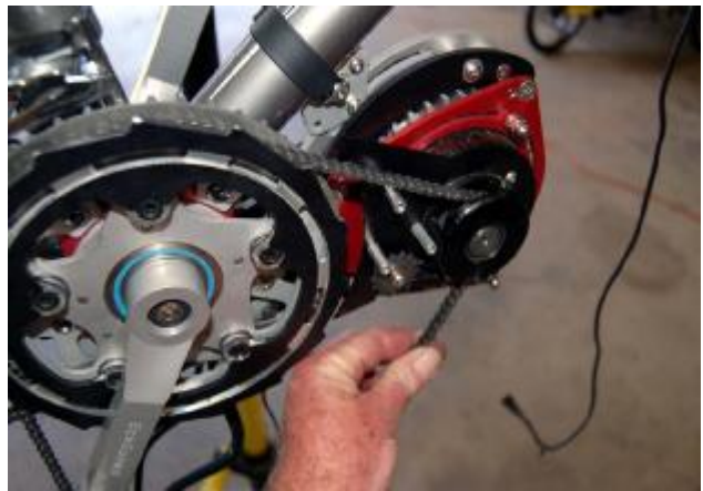
(14) Installing Motor Chain
