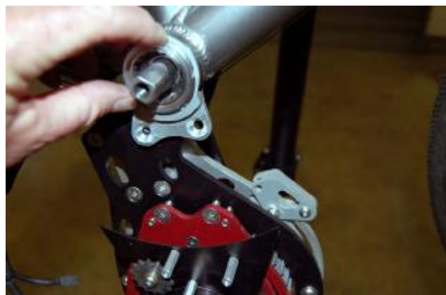
(8) Installing Right Lock Nut . Preparing to Re-attach Right Ring.
