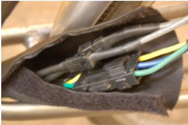
Wiring wrapped in Optional Velcro enclosure
