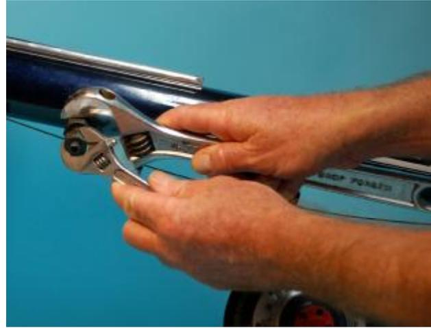
(5C) Wrench Type Rivet Nut Tool
