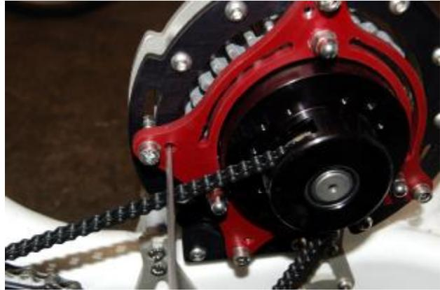
(8D) Using Set Screws to Align Motor Chain
