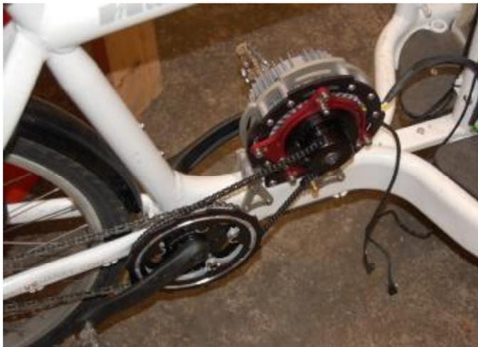
**(8) Installing the Motor Chain**
