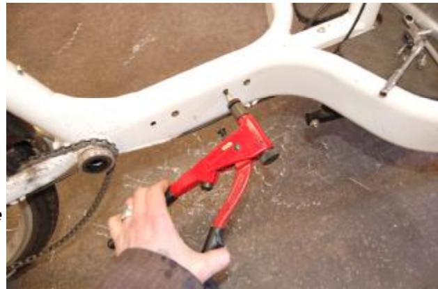
(5D) Lever Type Rivet Nut Tool
