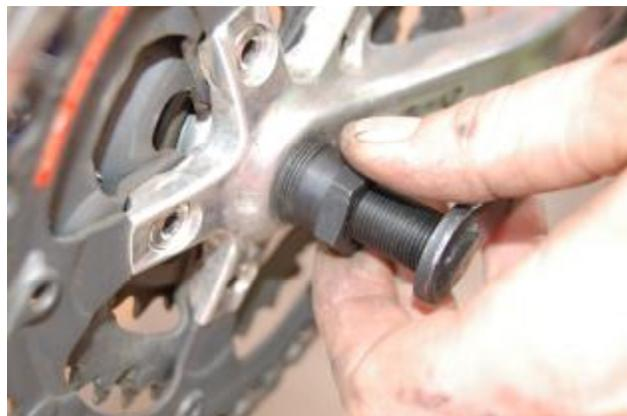
(2) Removing Crank with Crank Puller
